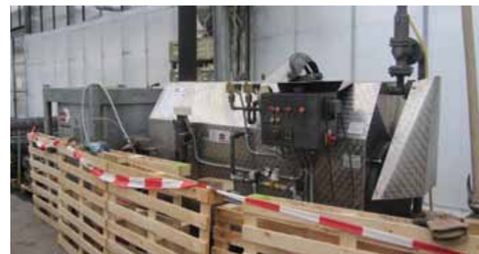
The tables are stacked and moved into the retrofitted container for the steam treatment. The mobile steamer (right) provides the necessary steam.
