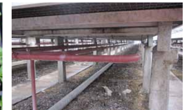
Heating is underneath the table and the wire-mesh covered with MayPex®. Keeping all surfaces clean, especially underneath the tables, is very important.
