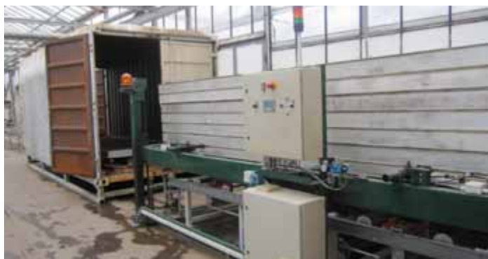
The tables are stacked and moved into the retrofitted container for the steam treatment. The mobile steamer (right) provides the necessary steam.
