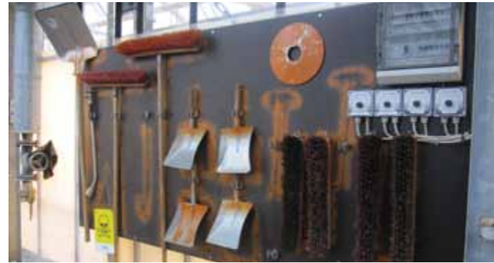
Every area uses a different color so equipment will find its way back easier and has its spot.
